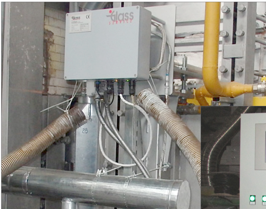
Radar glass level installed
