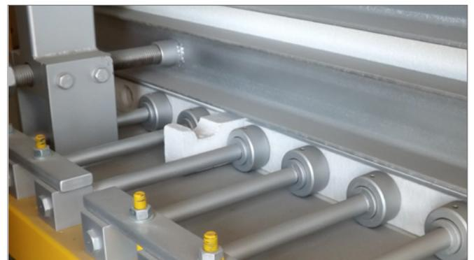
The burners are manufactured in special high temperature resistant steel.
