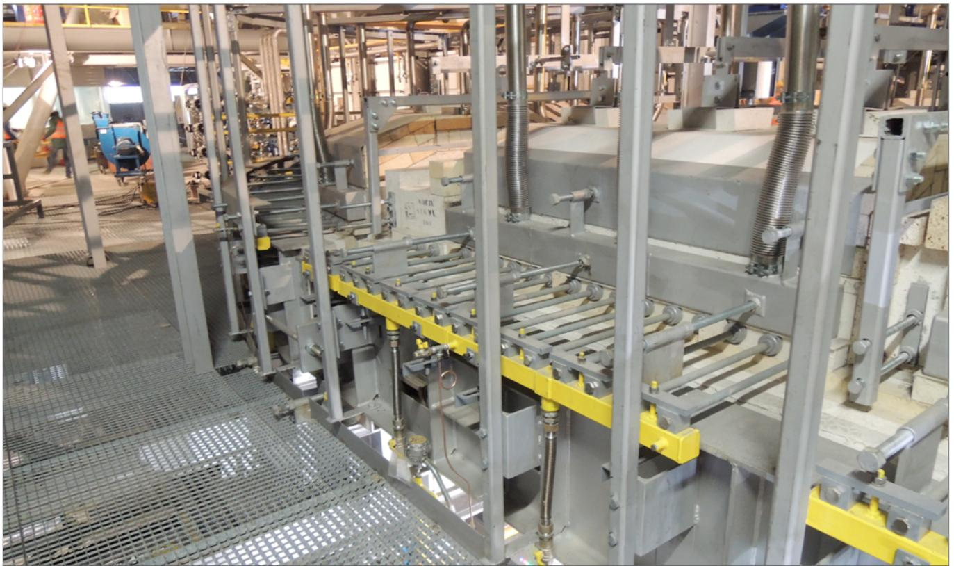
Glass Service developed the forehearth and distributor burner technology along with the necessary manifolds and mountings for the forehearth casing.
