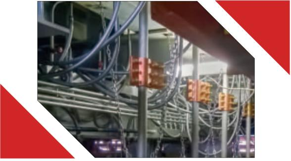
When installed to increase the furnace output, the booster can normally provide an additional 30% over and above the glass melted by the fossil fuel firing. Note that electric boosters are recommended in colour glass furnaces (green, amber, etc.) to maintain bottom temperature.
