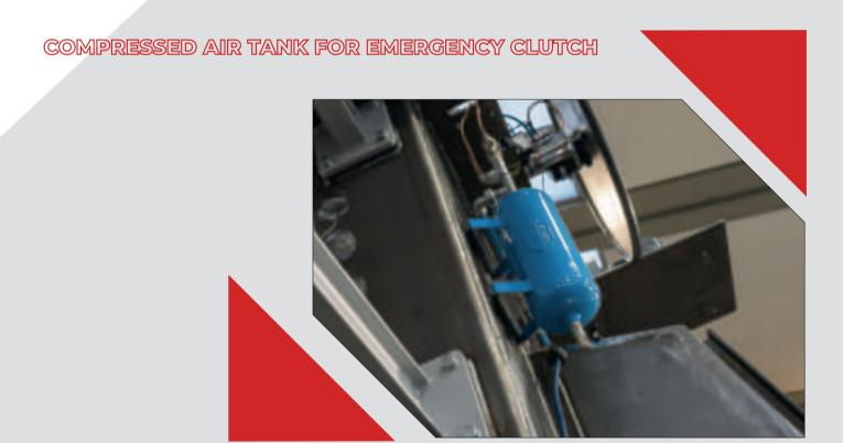
If the main compressor on-site fails, the Compressed Air Tank functions to provide the necessary amount of pressurized air to activate the clutch and allow for manual movement of the hand wheel. The system also includes a check valve, that prevents pressure drops in the tank once the main line cuts off the service.
