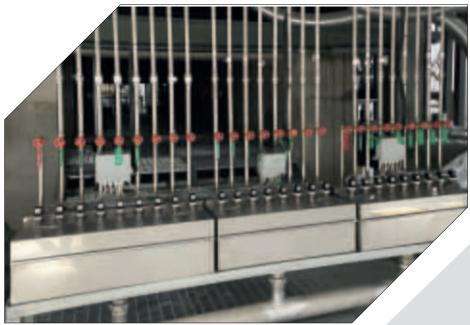
Each booster has a dedicated water cooling circuit to provide cooling water to the electrode holders using a special flow control and monitoring system designed by Glass Service.
