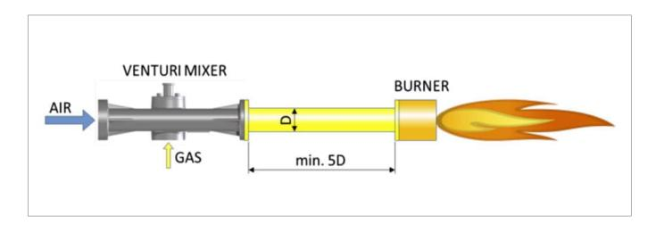
As shown in the image below the venturi mixer can be installed in symmetrical configuration and, according to the gas arrival line, has interchangeable gas entrance.
