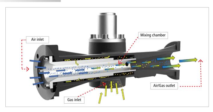
The energy of air passing through the venturi throat generates a depression with a consequential suction effect that forces gas to exit from the gas nozzle. The air/gas mixture then recovers pressure in the mixing chamber at the expense of velocity of the flow. The correct amount of gas is controlled by the pin regulation valve.
